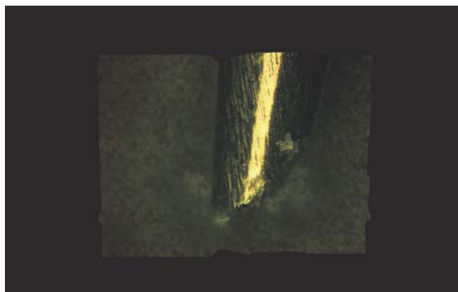
Figure 72. The point of tungsten needle seen through an optical scanning microscope. The point is 120 \mu\text{m} in diameter; 5000 \times magnification.
